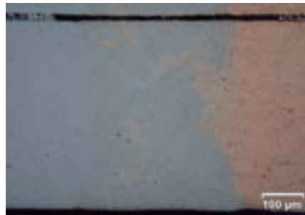
Polished sample of weld seam of copper-steel-combination
