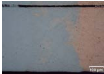
Polished sample of weld seam of copper-steel-combination
